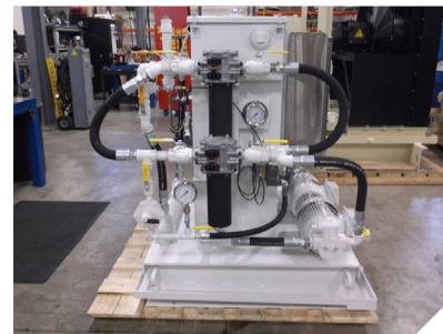
Hydrodynamic lubrication system
