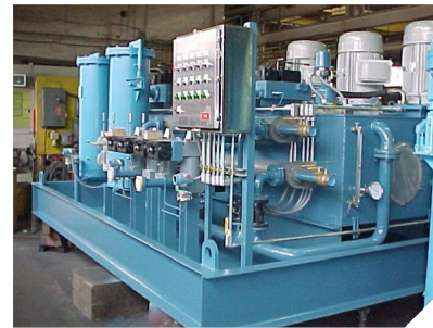
Hydrostatic lubrication system
